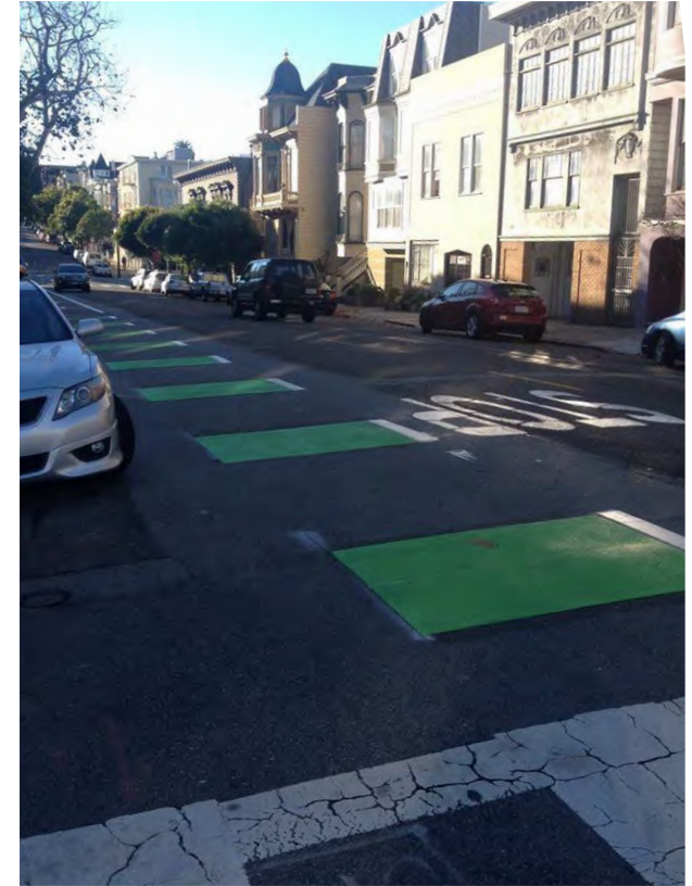
A San Francisco example of an intersection approach treatment that alerts cyclists and drivers to upcoming stop signs and conflict points. SOURCE: SFMTA LIVABLE STREETS
