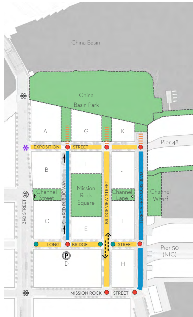
FIGURE 2.4.1 Vehicular Circulation Network Diagram illustrating vehicular movements, paseos, traffic signals, and stop control across the site. Refer to Chapter 4 for specific street controls, and to the Infrastructure Plan and Transportation Plan for details.
