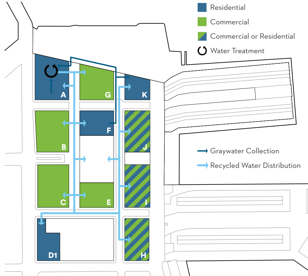
FIGURE 2.4: Graywater Collection and Reclaimed Water Distribution Infrastructure
