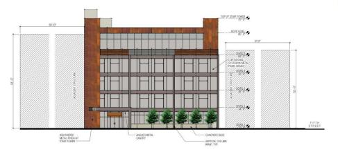
Figure 7: Proposed North Elevation
