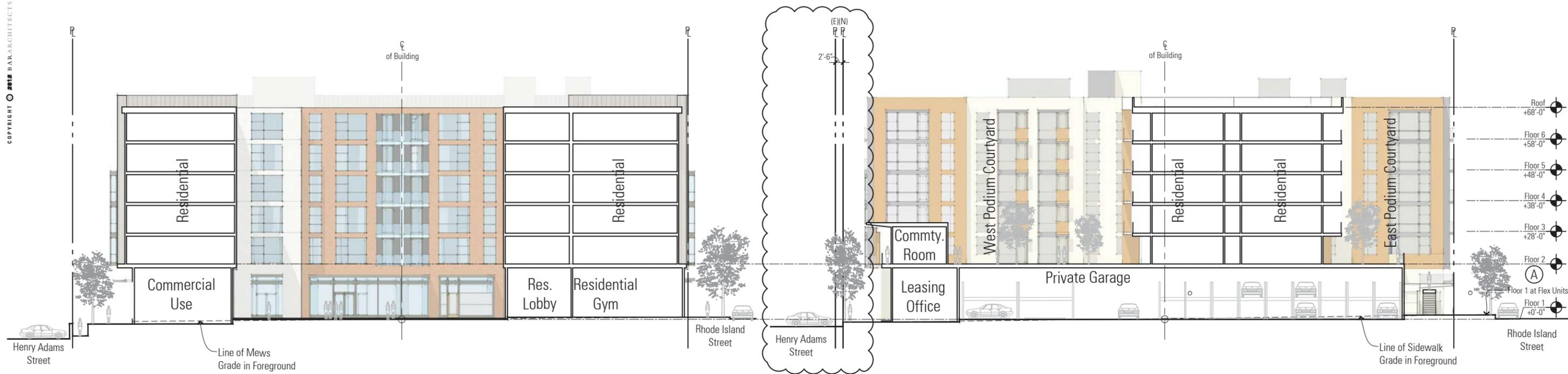
**Section B** Transverse Section of North Building Looking North
