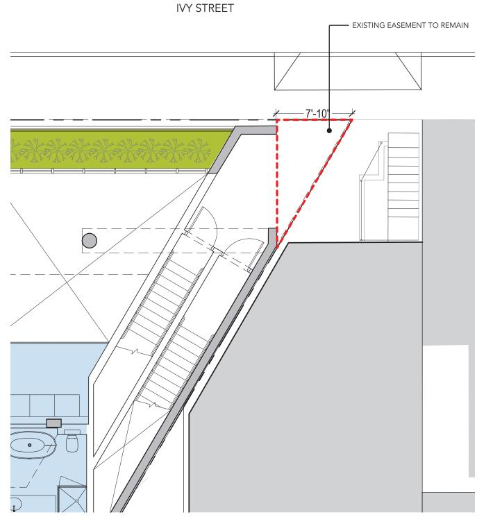
PROPOSED GROUND FLOOR PLAN AT NORTH-EAST EASEMENT
