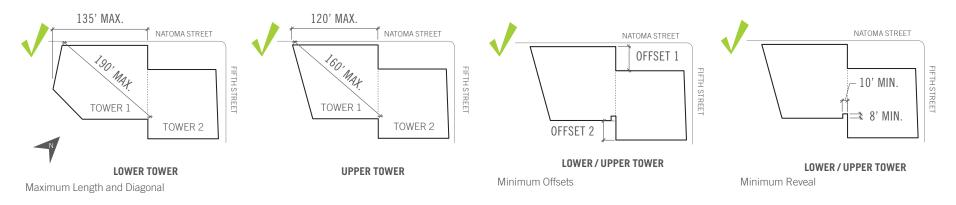
Fig. 5.4.2b Two-Tower Floorplate Examples
