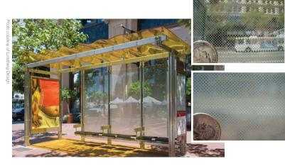
ABOVE: The City's new bus shelters designed by Lundberg Design use a subtle frit pattern to indicate the barrier. This design, called "SF Fog," is effective in alerting both people and birds to the glass. INSETS show how the frit pattern is more dense at the bottom and dissipates like the City's fog at the top.
