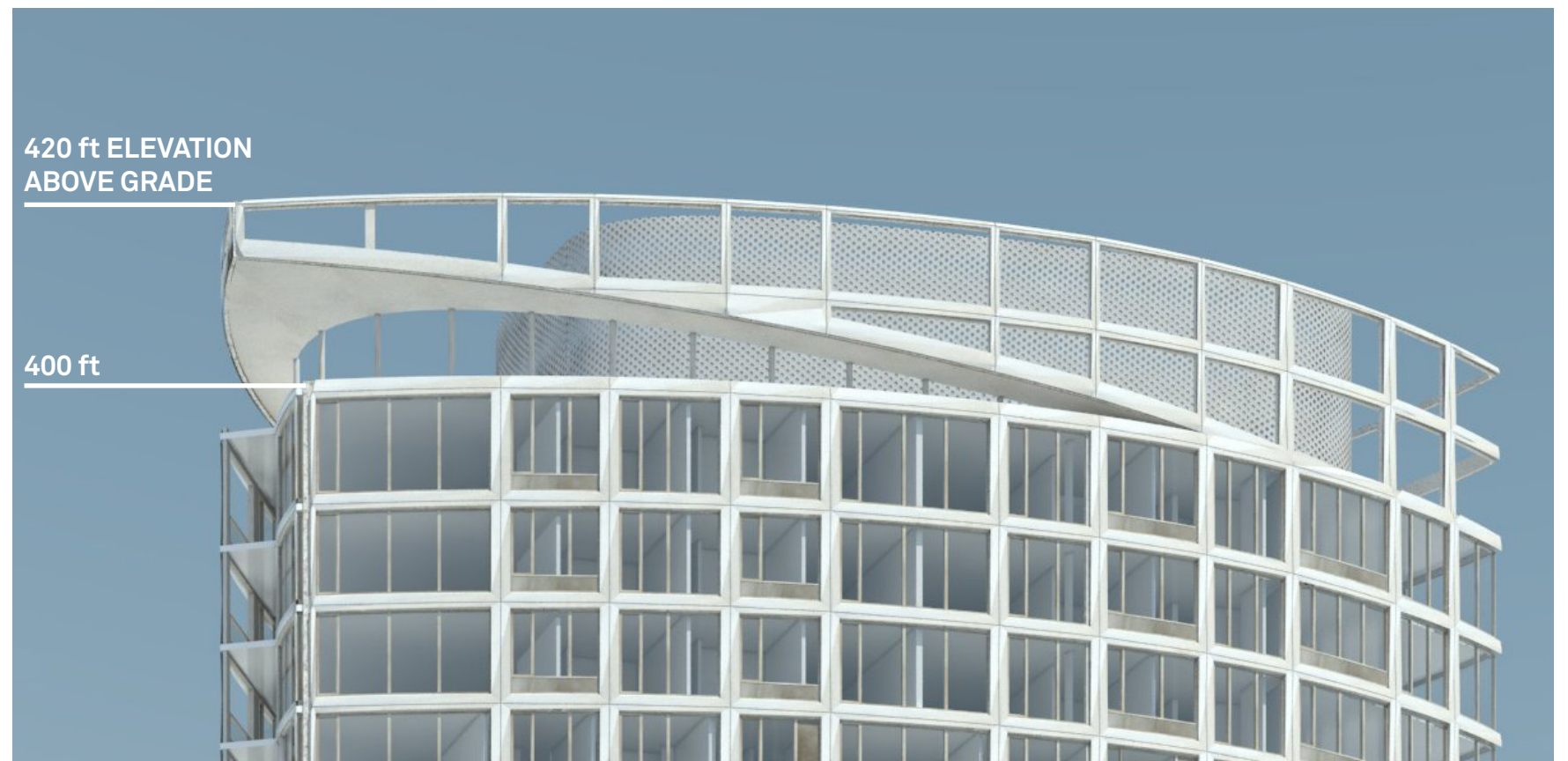
EXTENSION OF TOWER FACADE TO COVER ROOFTOP EQUIPMENT AND UNIFY SKIN DESIGN
