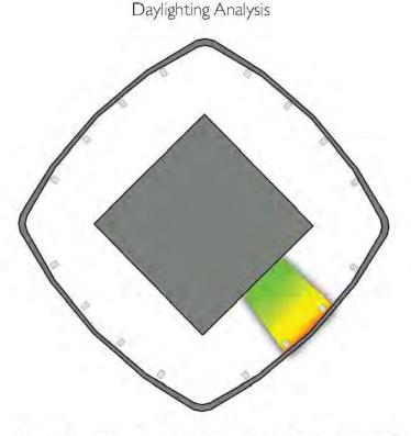
Daylight analysis can inform façade design and optimization of daylight controls for artificial lighting systems
