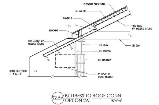
Figure A14 - Option 2A -Buttress to Roof Connection
