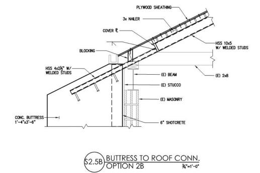
Figure A15 – Option 2B –Buttress to Roof Connection
