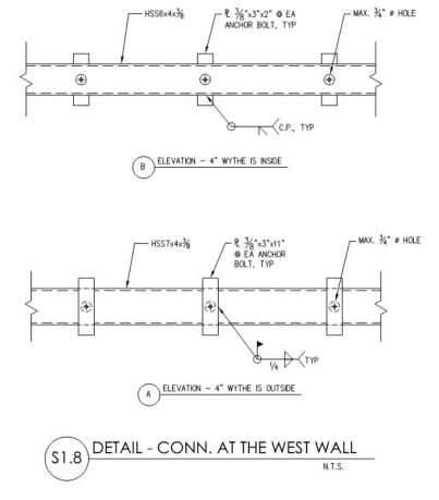
Figure A8 – HSS to HCT Masonry Wall connection
