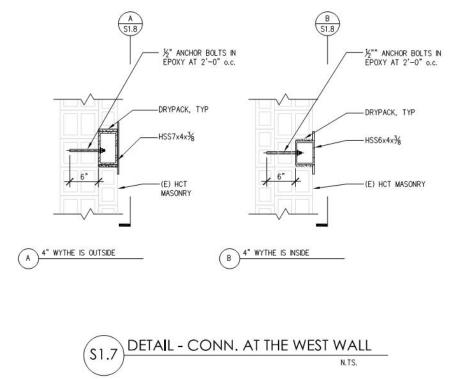
Figure A7 - HSS to HCT Masonry Wall connection
