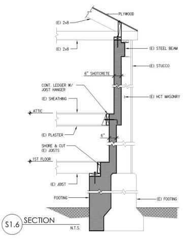
Figure A6 – Options 1, 2A, and 2B - Section at Attic Area
