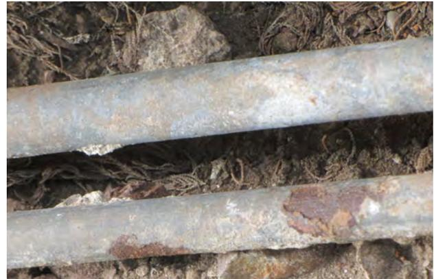
Figure 5.63: Corroded piping in crawlspace.
