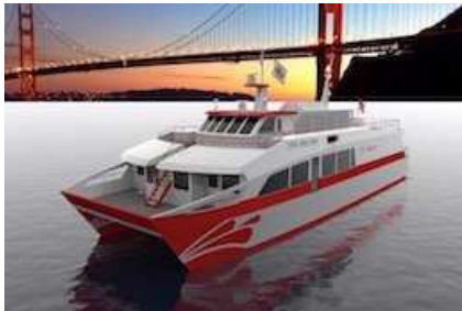
SF-BREEZE is a zero emissions concept ferry, set to be powered by a hydrogen fuel cell.
