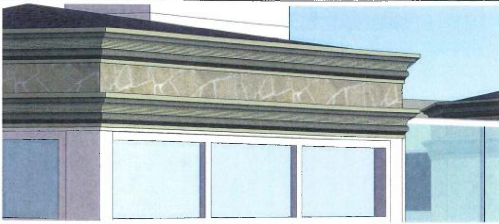
CLOSE-UP OF DOUBLE CORNICE & TOP FLAGSTONE VENEER FASCIA AT ROOF MONITORS & TERRACE
