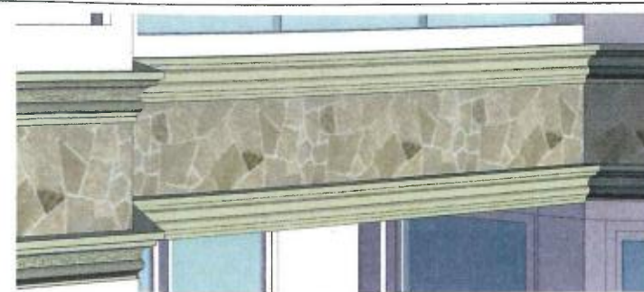
ENLARGED VIEW OF TOP CORNICES & STONE FASCIA
