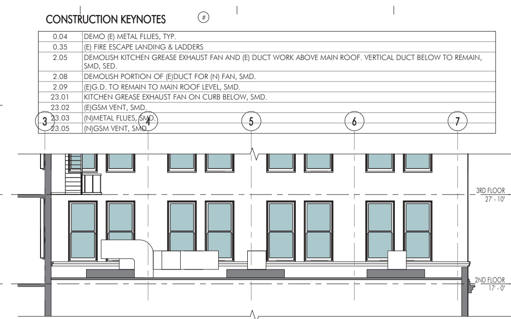
3 2ND FLOOR ROOF SECTION - LIGHT COURT 3/16" = 1'-0"
