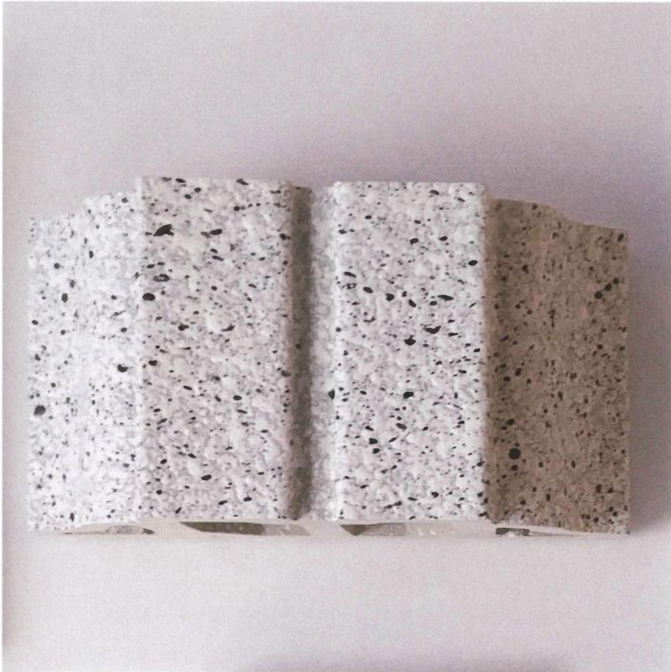
Terra cotta wall panels with textured surface (Photograph of Project Material Sample: to be finalised) Color and tone to be similar to existing grey granite
