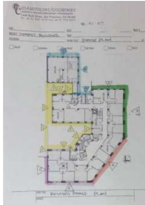
Giampolini Courtney took scores of photographs of terra cotta failure and deterioration, and the steps of repair. The exterior was divided into vertical segments or drops, and the work moved around the building in a generally clockwise direction. At least once each year, the contractor adjusted the phasing plan. (All photographs and drawing by Giampolini Courtney.)
