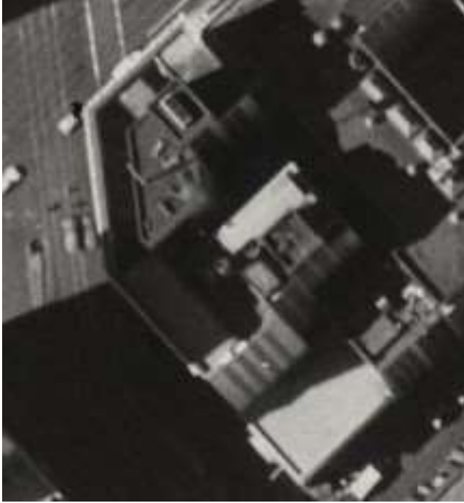
Left: Aerial view of the Hearst Building in 1938 shows the penthouse structures similar in shape to the 1968 leasing plan including the original 1911 residential unit, lobby and elevator machine room wrapped by a new set of structures/spaces. (David Rumsey Map Collection, San Francisco Aerial Views, Harrison Ryker, 1938.)
