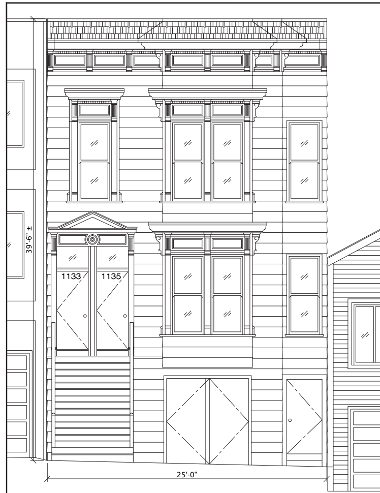
1 FRONT/WEST ELEVATION - EXISTING 1/4" = 1'-0"
