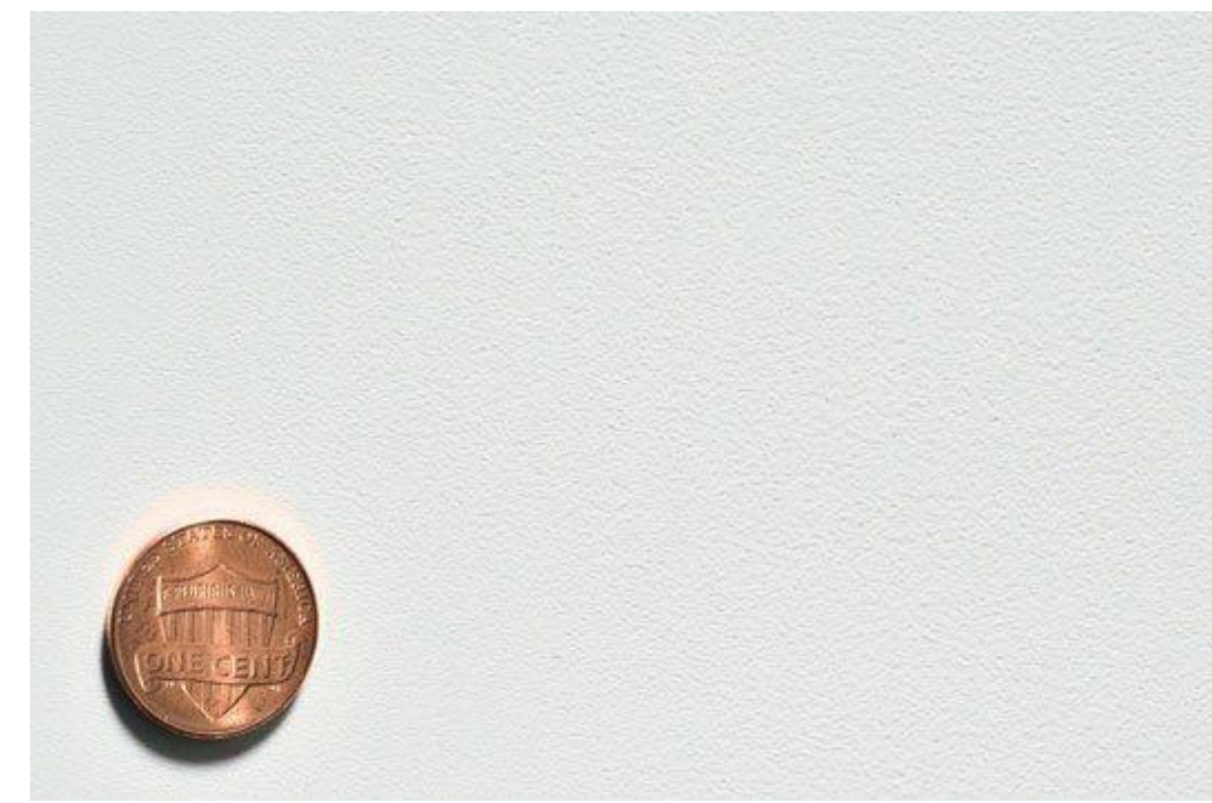
Synthetic, Acrylic-Based Stucco Ultra-Smooth Finish
