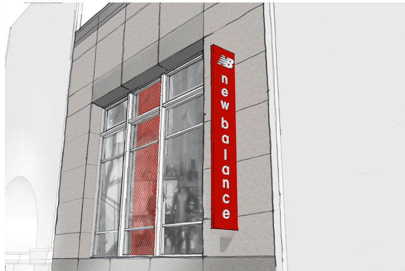
1 INTERNALLY ILLUMINATED PUSH THROUGH LETTERS ON OPAQUE BACKGROUND
