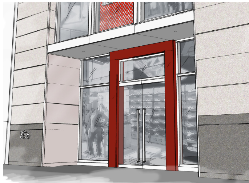
2 METAL BRAKE FORMED ENTRY PORTAL
