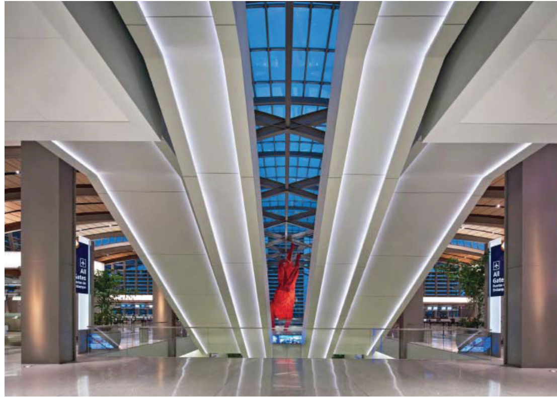
Lighting: LED Cove Lighting
