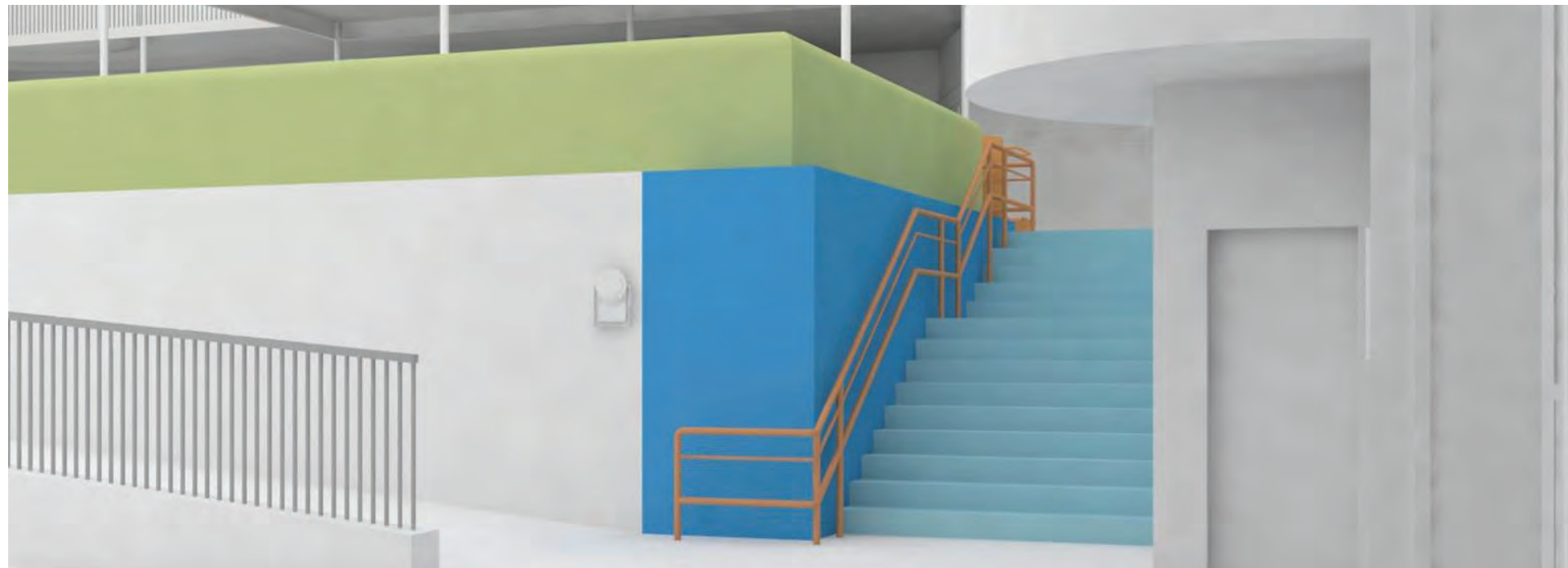
View of proposed lift and new stair. Lift shown in the up position (Terrace Plaza position)
