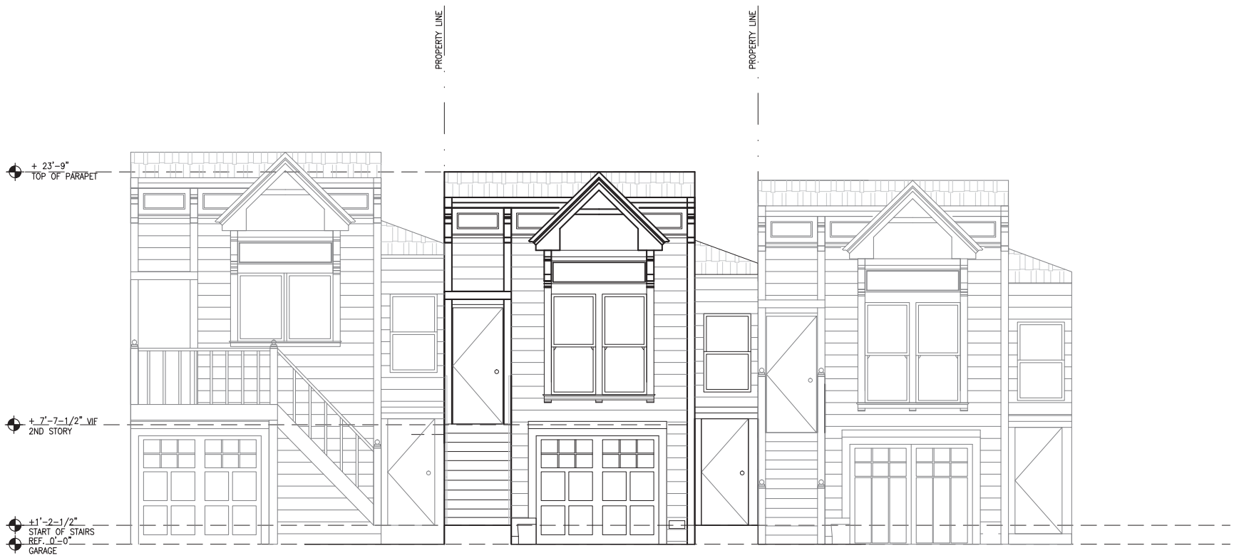
1 EXISTING WEST ELEVATION A2.01 1/4" = 1'-0"
