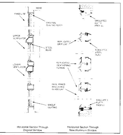
Figure 6. Sections of original and replacement windows. Drawings: Bruner/Cott and Custom Window.
