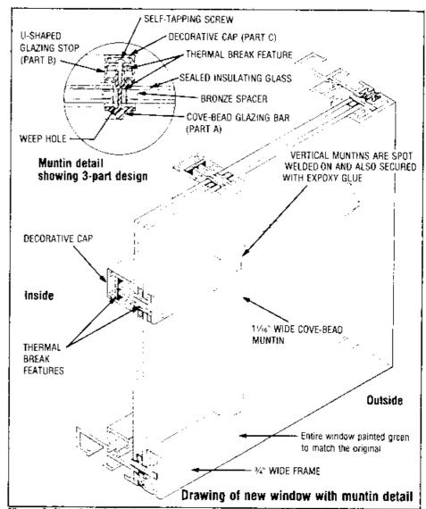
Figure 3. Drawing of the aluminum replacement windows shows how the covebead muntin profile of the original steel windows was closely matched in the integral muntin system designed for the aluminum replacement window. A series of spacers and gaskets were used as the principal means of obtaining a thermal break in the window for energy purposes. Drawing: Peter Charles
