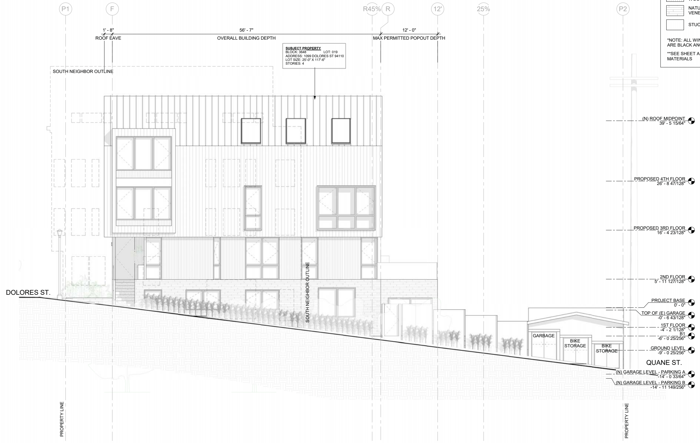
1 PROPOSED SIDE (SOUTH) ELEVATION 3/16" = 1'-0"
