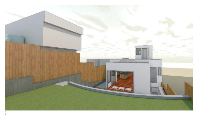
> Design following 5.8.18 RDAT meeting with a passive solar venting column with south facing skylights and north facing exhaust vents >
