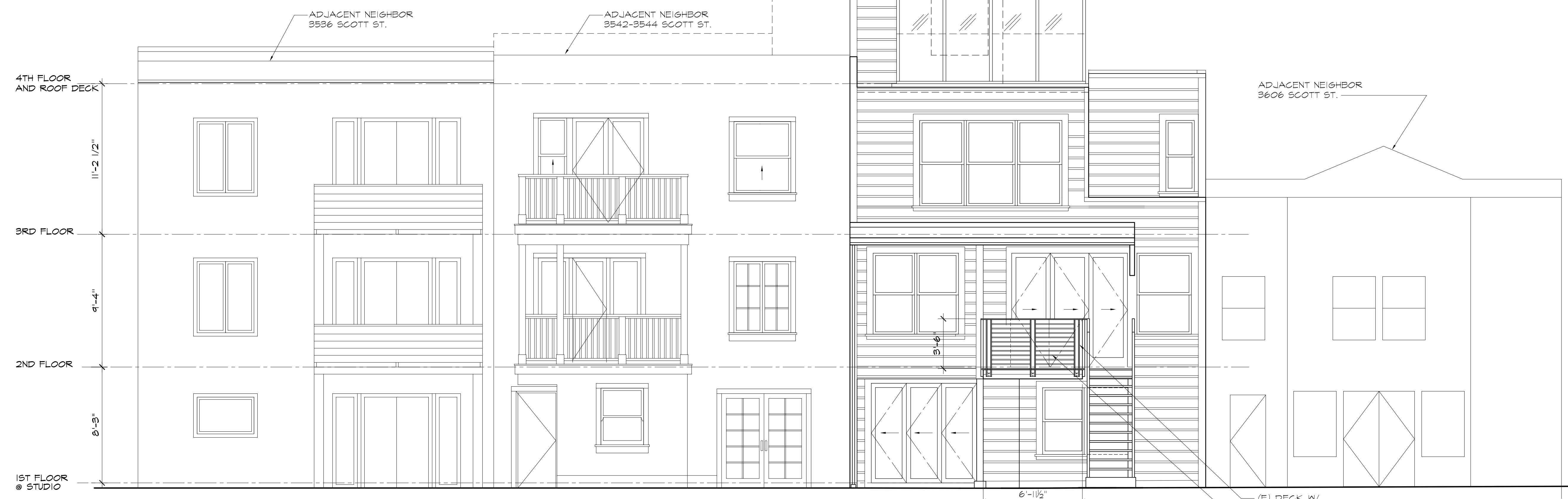
REMODELED EAST ELEVATION SCALE 1/4"=1'-0"
