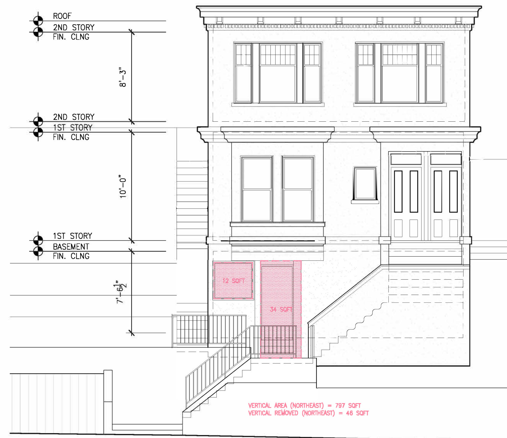
1 EXISTING EAST ELEVATION SCALE: 3/16" = 1'-0"
