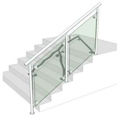
12 GLASS GUARDRAIL REFERENCE "A" 6" = 1'-0"
