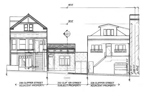
CLIPPER ST (E) EXTERIOR ELEVATIONS
