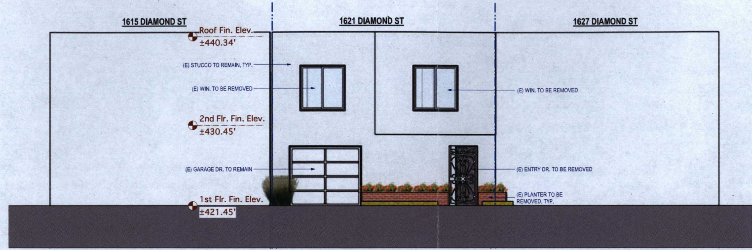
Existing Front Elevation(West) 1/4" = 1'-0"
