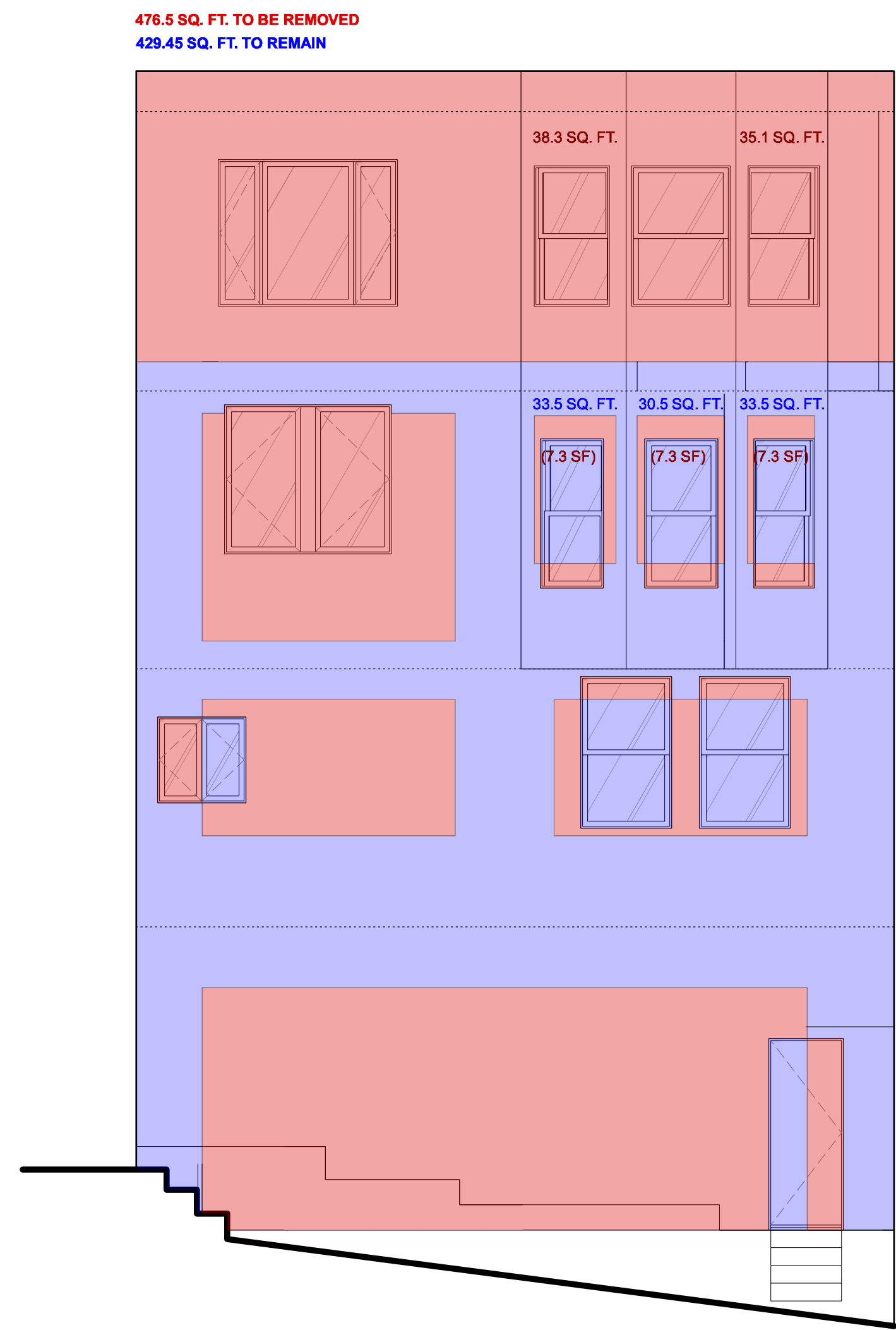
2 EXTERIOR ELEVATION - REAR (EAST) - EXISTING/DEMOLITION Scale: 1/4" = 1'-0"
