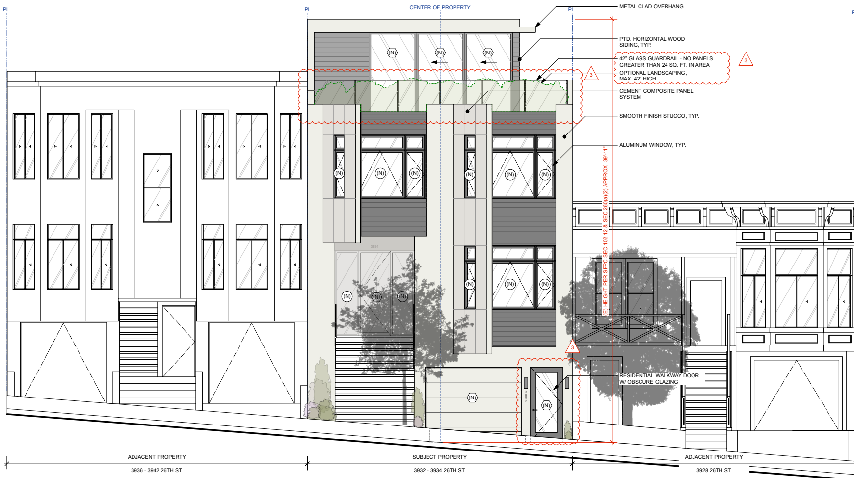
2 SOUTH (FRONT) ELEVATION - PROPOSED Scale: 1/4" = 1'-0"
