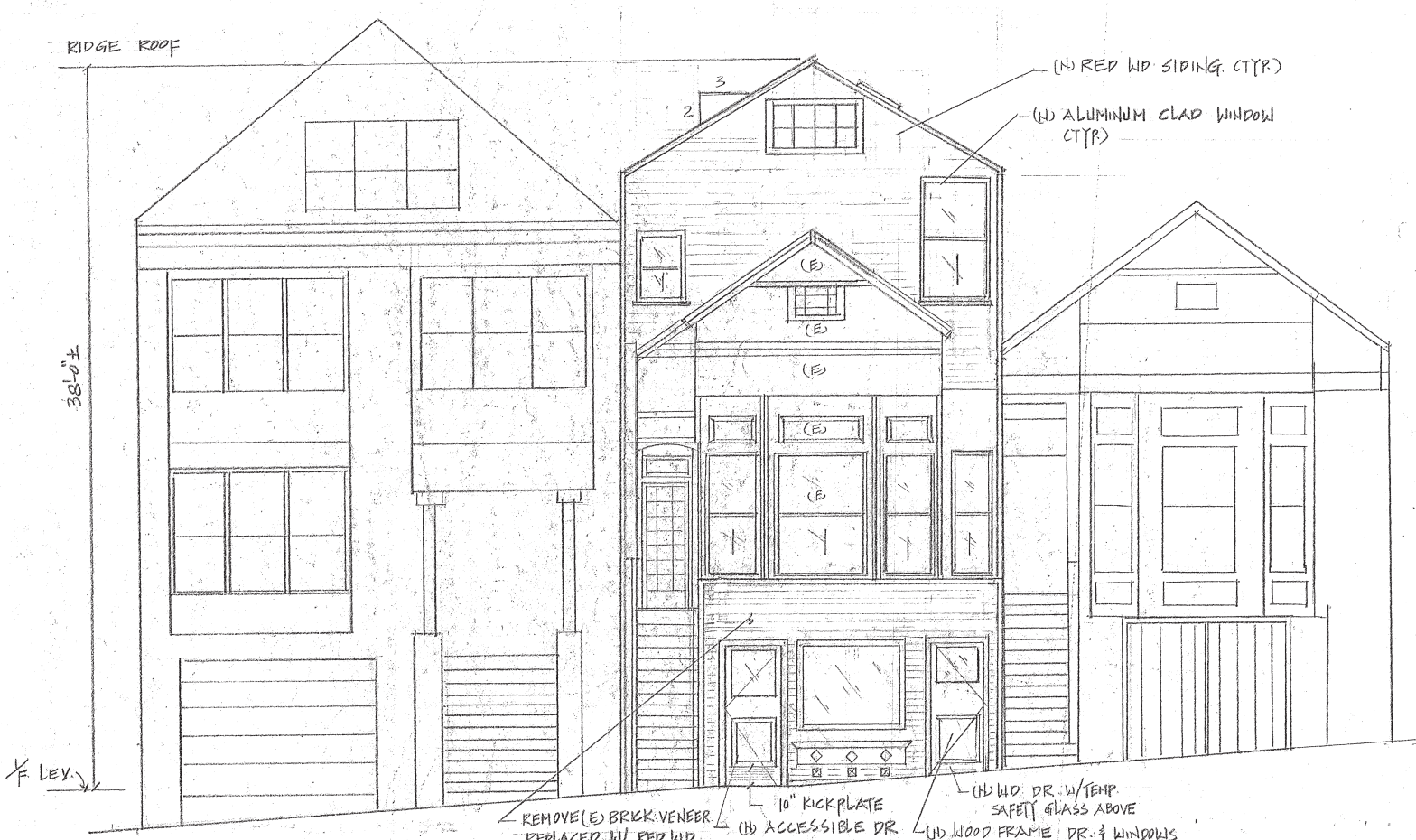
EXISTING ADJ. FRONT ELEVATION H 4-13-9 1/4" = 1'-0" PROPOSED FRONT ELEVATION H 4-14-3 1/4" = 1'-0" EXISTING ADJ. FRONT ELEVATION H 4-14-7 1/4" = 1'-0"
