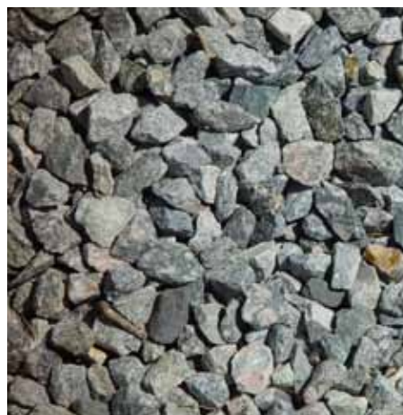
1 1/2" Diameter Rough Crushed Gravel at Tree Well
