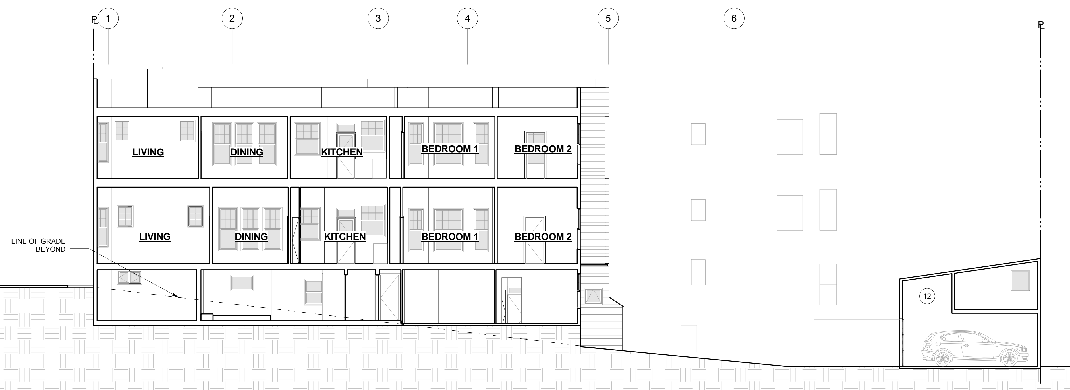
2 (E) SITE SECTION @ CL OF BUILDING 1/8" = 1'-0"
