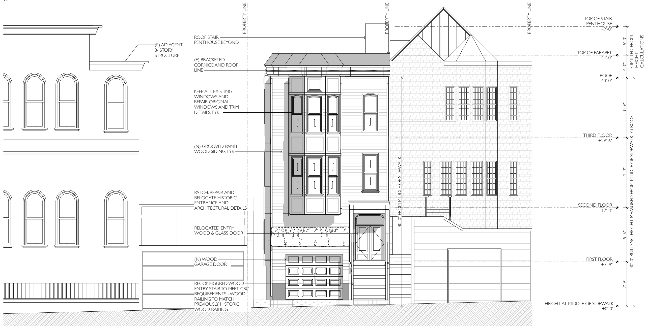
1 PROPOSED SOUTH (FRONT) ELEVATION
