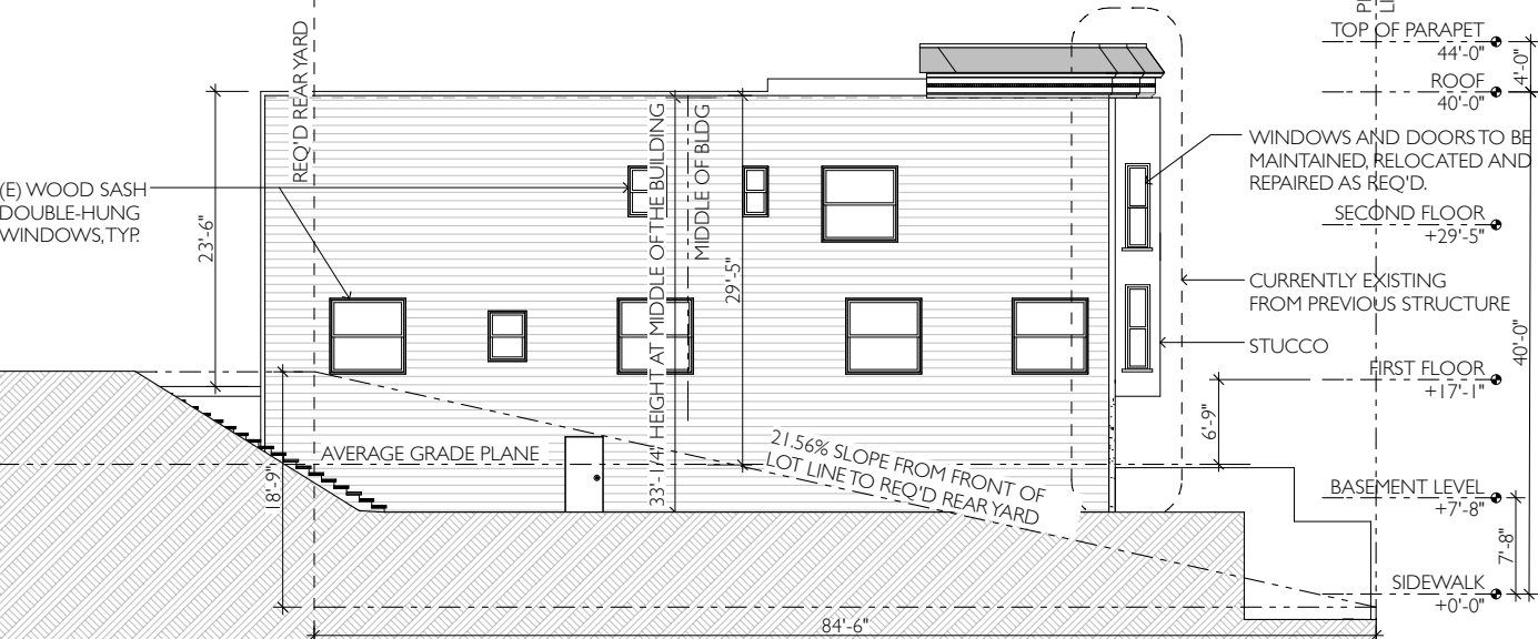
6 PREVIOUSLY EXISTING WEST ELEVATION SCALE: 1/8" = 1'-0"
