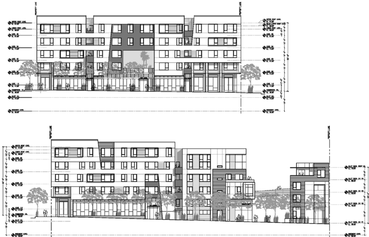
Figure 10 – 9th Street Elevation (top) & Howard Street Elevation (bottom, showing Natoma Street Driveway Option)
