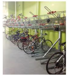
Mechanical Lift-assist & U-lock Double Decker Bicycle Racks
