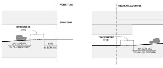
FIGURE 5.6.1: Driveway Slope and Top Transition Strip
