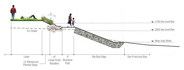
FIGURE 3.8.5: Illustrative Shoreline Section 2 Note: All dimensions and elevations are illustrative only.
