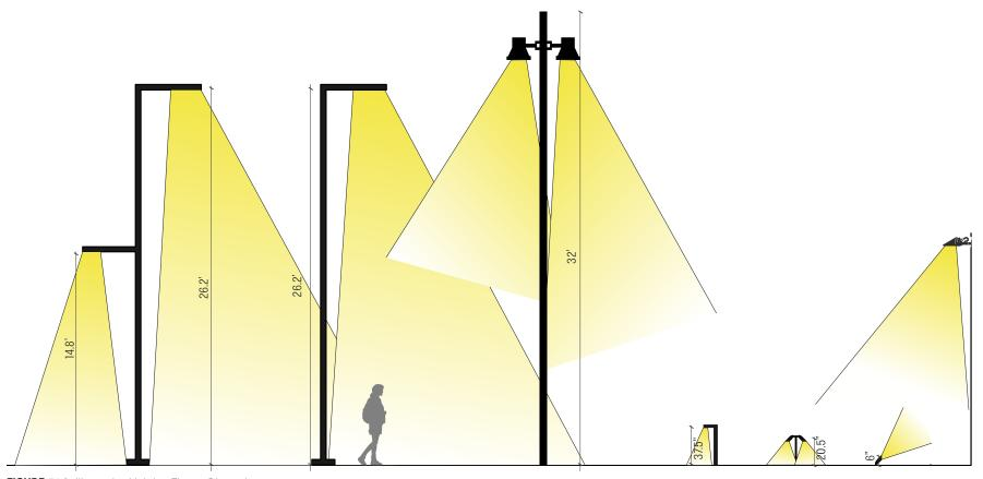
FIGURE 7.1.3: Illustrative Lighting Fixture Dimensions
