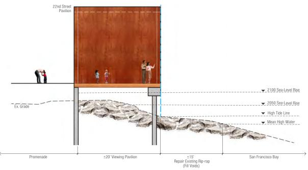
FIGURE 3.8.8: Illustrative Shoreline Section 3 Note: All dimensions and elevations are illustrative only.
