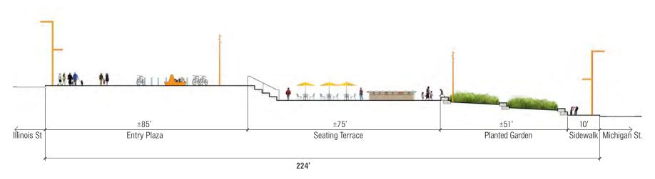
FIGURE 3.10.2: Illustrative 20th Street Plaza Section Note: All dimensions and elevations are illustrative only.
