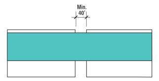
Partial Floorplate Horizontal Building Connector - Plan
