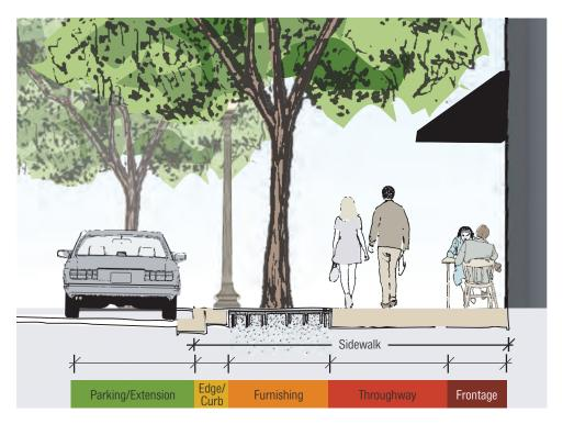
FIGURE 4.3.2: Sidewalk Zones Section
