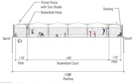
FIGURE 3.12.2: Illustrative Section A-A: Active Recreation Note: All dimensions and elevations are illustrative only.
