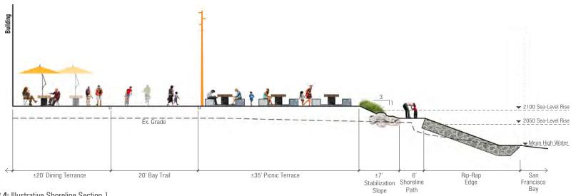
FIGURE 3.8.4: Illustrative Shoreline Section 1 Note: All dimensions and elevations are illustrative only.
