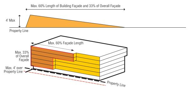
FIGURE 6.10.3: Aggregated Occupiable Projections
