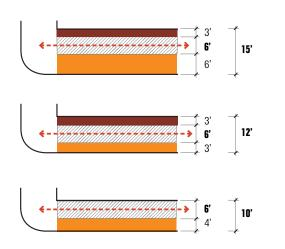
FIGURE 4.3.3: Effective Sidewalk Width – 6' Minimum Throughway Zone
