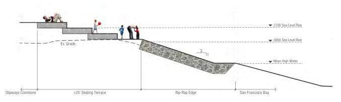
FIGURE 3.8.9: Illustrative Shoreline Section 4 Note: All dimensions and elevations are illustrative only.
