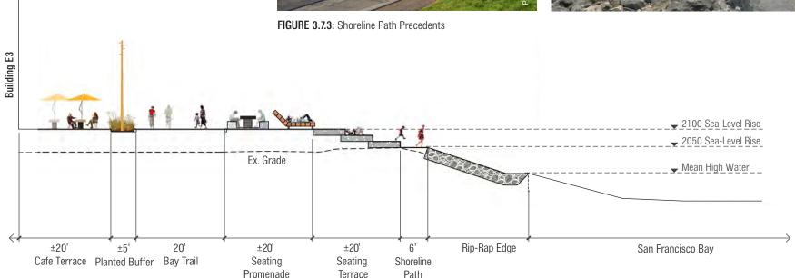
FIGURE 3.7.2: Illustrative Waterfront Promenade Section Note: All dimensions and elevations are illustrative only.
