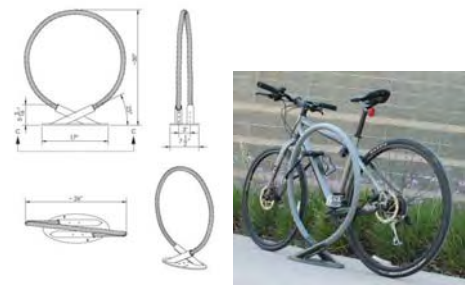
NOTES: 1. ECOFLEX BIKE RACK 2. LOCALLY SOURCED AND MANUFACTURED 3. MADE FROM RECLAIMED, COATED STEEL CABLE: RESISTANT TO CUTTING BIKE RACK
