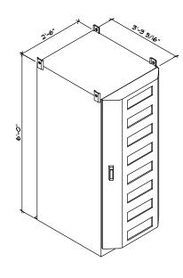
ISOMETRIC VIEW OF POWER AND BATTERY CABINET
