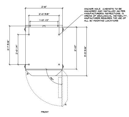
BOLT DOWN PATTERN FOR POWER AND BATTERY CABINET
