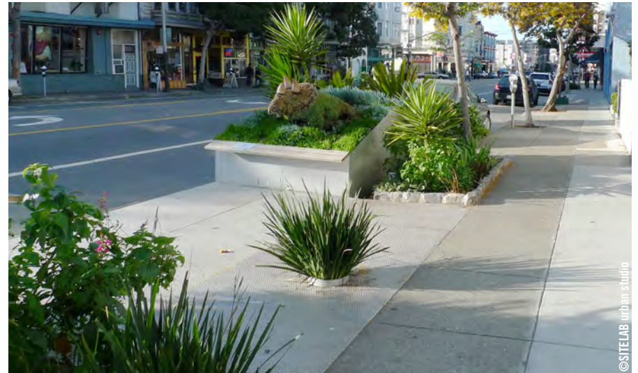
Permeable paving, planters, and drought resistant planting can contribute to rain-harvesting, ground water recharge, and reduce heat-island effect. Valencia Street / San Francisco, CA
