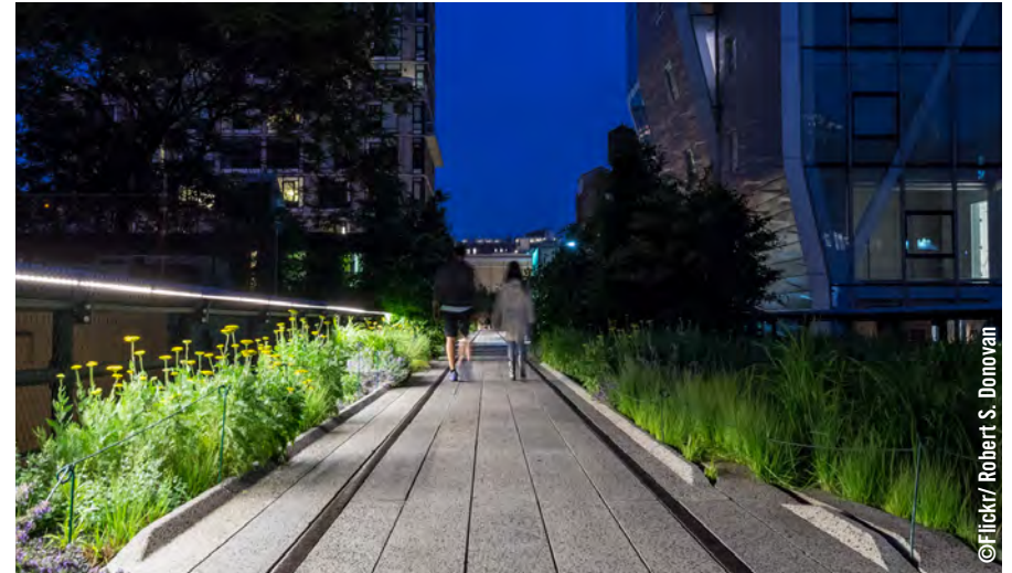
Open Space Pathway Lighting – downlighting integrated in railing
