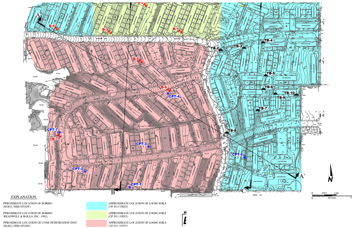
Soil boring site plan: Up to 5' of loose soils are located at the portion of site east of Santos Street. (Figure 1.6)
