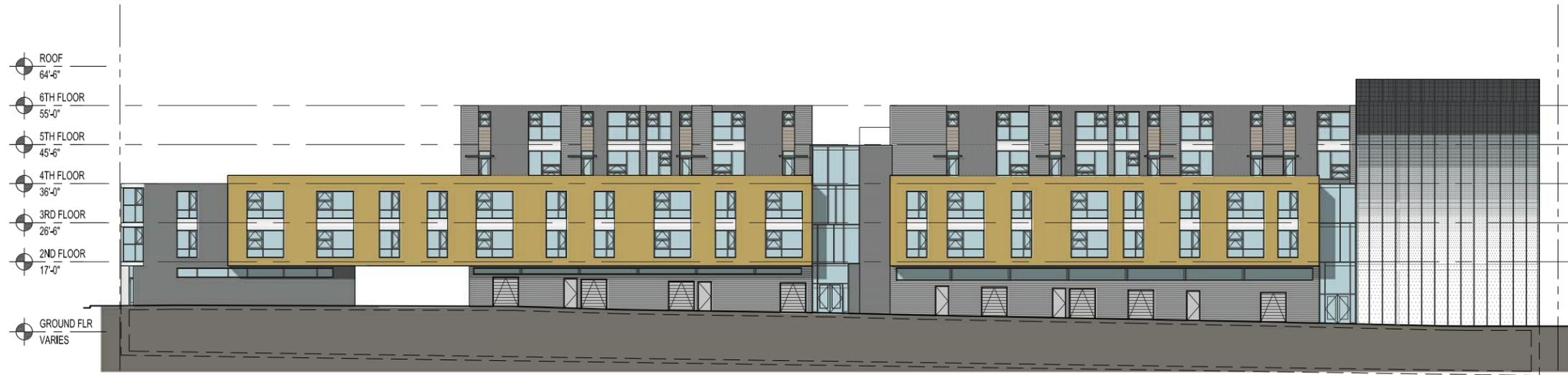
NOTE: INDIVIDUAL GLAZING PANELS LARGER THAN 24 SF SHALL BE FRITTED (TO COMPLY W/ SFPC SECTION 139).
