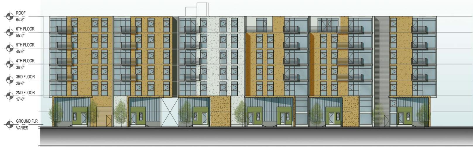
BUILDING 7 SOUTH ELEVATION (BUILDING 6 NORTH ELEVATION SIMILAR) 2
