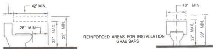
(a) WATER CLOSET IN ADAPTABLE BATHROOMS
